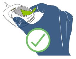
NOTE! The correct orientation of the Coala when placing it into the Coala Charge Station. Do not use force or press straight down on to the Coala when placing it into the Charge Station. For maximum electrical safety, the Coala cannot be used while charging. Coala Charge Station and connected wall adapter are IT type equipment and do not carry the type BF (Body Floating) medical electrical safety rating that the Coala does.
