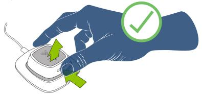
Do not use excessive force when lifting the Coala out of the Charge Station as this will damage the device
