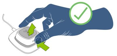
between the Charge Station (small USB plug) and Wall Adapter (large USB plug). Connect the Wall Adapter to the power outlet.
